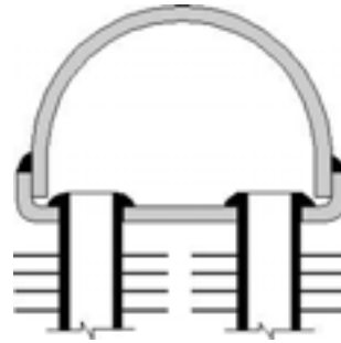
HP Series heater shape. Available in one, three, five and seven pass configurations depending on model. Pressure up to 400 PSI. Operating pressure on select models.
